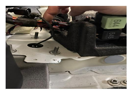
13. SET THE REAR MOUNTS IN PLACE PULLING THE SHOCK WIRES THROUGH THE CENTER HOLE OF THE MOUNT TOWER. JUST START THE NUTS FOR THE REAR MOUNT. DO NOT FINAL TIGHTEN ANY NUTS OR BOLTS UNTIL THE WHOLE ASSEMBLY IS INSTALLED. PLUG IN THE REAR SHOCK WIRES AND LOCK TABS.
