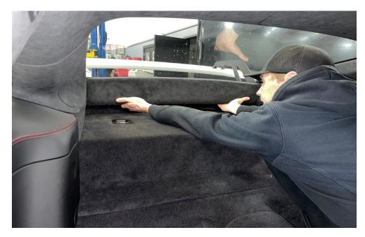
5. REMOVE REAR ANCHOR POINT TRIMSWITH A PRY TOOL.
