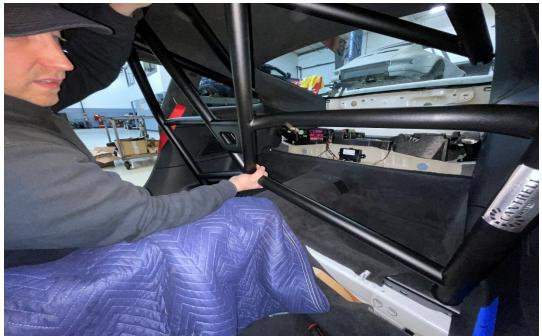
16. ALIGN AND START THE REAR INTERLOCK ALLEN BOLTS. AGAIN, DO NOT FINAL TIGHTEN YET. JUST THREAD JUST SHORT OF FINAL.
