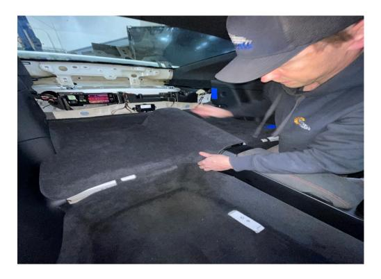
9. FOLD THE BACK CORNERS OF THE MAIN CARPET DOWN TO EXPOSE WIRE HARNESS LOOMS AND CROSSMEMBER BOLTS.
