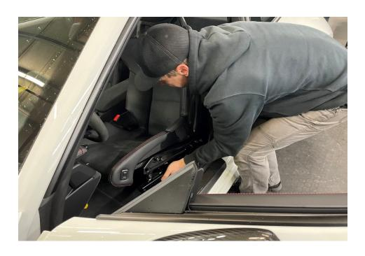
3. BEFORE REMOVING ANY CARPET OR TRIM, LAYOUT SOME BLUE PAINTERS TAPE FOR MARKING OF HOLE CUT LOCATIONS. PLACE THE EDGE OF TAPE ALONG THE SIDE OF THE LOWER CARPET AS IT RESTS AND ANOTHER ON TOP OF THE LOWER CARPETJUST ABOVE THE CROSSMEMBER THAT IS BELOW IT. (LIFT CARPET AND TAKE A PEEK FOR REFERENCE) PLACE ANOTHER TWO STRIPS FOR THE REAR HOLES AT THE BACK EDGE OF SIDE PANEL AND THE CARPET WHERE IT MEETS THE SIDE PANEL. ON ALL FOUR LOCATIONS MAKE A SHORT MARK IN LINE ACROSS BOTH PIECES OF TAPE.
