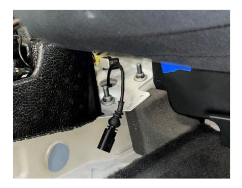
27. BRING LOWER CARPET SECTION INTO THE ROLL BAR THROUGH A LOWER OPENING. START WORKING IT BACK FORWRD UNDER THE LOWER BAR INTO POSITION. FOLD THE SIDES TO BRING AROUND THE MAIN HOOP BASE. ALIGN THE PLASTIC CLIPS IN THE MIDDLE HUMP. USING YOUR FINGERS YOU CAN CHECK THE ALIGNMENT OF THE METAL CLIPS WITH THE METAL TAB ON THE BODY.
