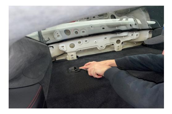
6. REMOVE UPPER CARPET PAD BY GRABBING THE LOWER MIDDLE AND MAKING A FOLD UP TO PULL OUT FROM THE SIDES.
