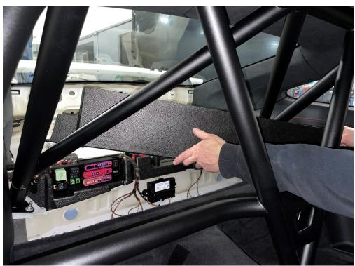
20. MEASURE FROM THE EDGE OF THE REFERENCE TAPE TO THE CENTER OF THE MAIN HOOP TUBE AND NOTE IT. THEN USING THE TAPE MEASURE, COMPARE THE CENTERLINE OF TUBE TO THE CENTERLINE OF THE MARK ON THE PERPENDICULER AXIS AND NOTE. USE THE SAME PROCESS FOR THE REAR CARPET.
