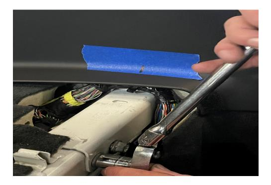
12. USE THE REAR MOUNTS TO MARK HOW MUCH TO TRIM FROM THE LOWER STYROFOAM HOLDER IN THE REAR. THIS CAN CUT IN PLACE OR FISHED OUT OF CAR FOR CUTTING.
