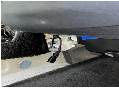
8. NOW REMOVE THE REAR LOWER CARPET COVER. THERE ARE METAL CLIPS ABOUT 5" IN FROM THE SIDES ALONG THE FRONT EDGE THAT RELEASE BY PULLING FIRMLY STRIAGHT UP. THE BACK EDGES HAVE VELCRO ATTATCHMENT POINTS. THE FRONT OF THE MIDDLE HUMP HAS PLATIC ARMS THAT EXTEND FORWARD AND HAVE CLIPS THAT PULL STRAIGHT UP.
