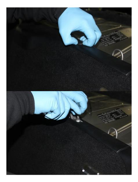
Remove top trim piece by removing the 1 screw below grab bar then pull/pry up working from one end to the other.
