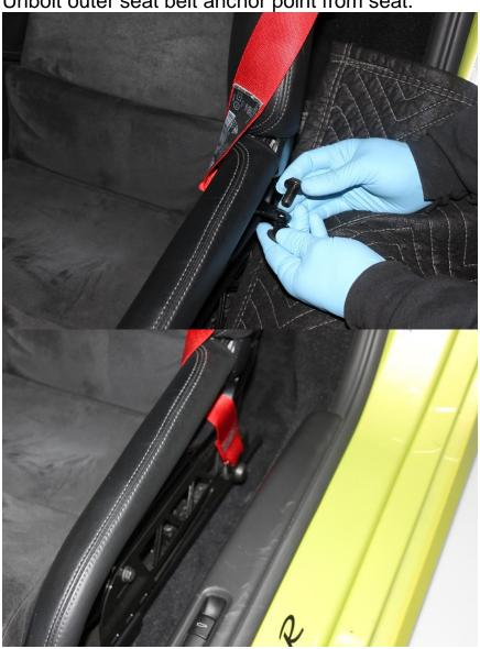
Remove floor front lower floor seat trim to access bolts for seat.
