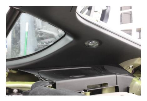
Install main hoop assembly again but do not final tighten. Be sure to put the two M8 washers between the seat belt guide pin and the body for correct
