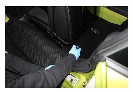
Unplug seat at large yellow connector by first releasing black lock tab, pulling it straight out.
