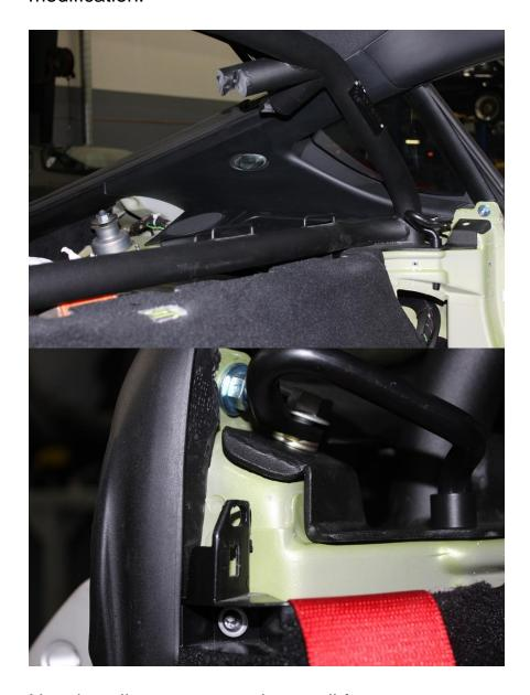
Next install rear stays and start all fasteners. Raise rear of car and set on jack stands to allow full droop of suspension. Then install new bolt for rear stays from the wheel well into the cabin and start nut. (Assistance from a second party will be helpful for this bolt.)
