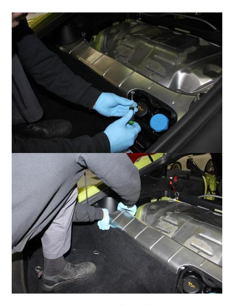
Remove upper grab bar at front of engine cover by pulling up rubber base trims to access bolts. PIC
