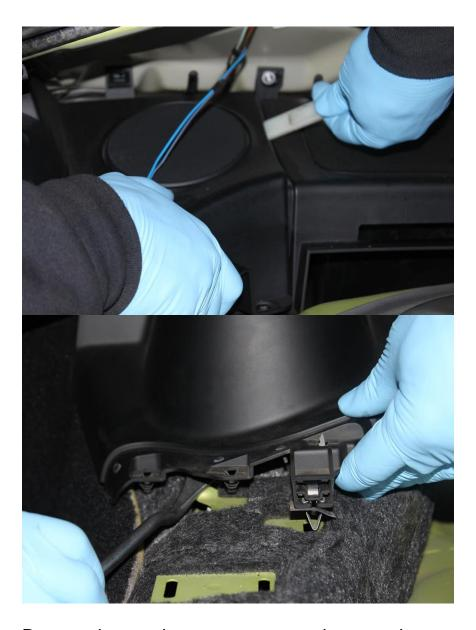
Door pocket sections now come out by removing the 4 remaining screws then prying at the clips around the seat belt area pulling them to the middle of the car.
