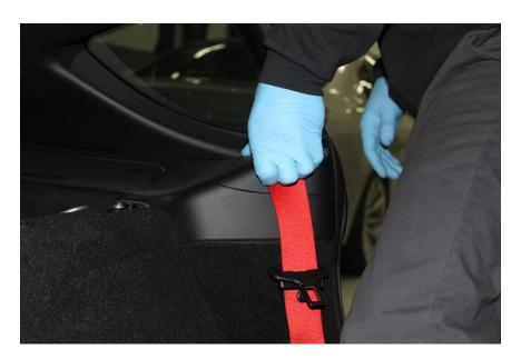
C pillar trim can now be removed by first removing screw at the lower front edge for each side. The trim piece can now be pried out by starting at the top hatch opening and pulling down. Unplug light then pull trim up and out.
