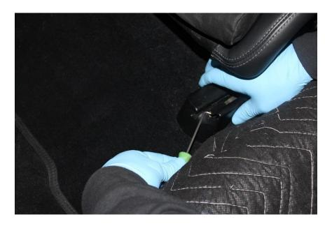
Unbolt the seats at the four points, then tilt seat back to access plug below.
