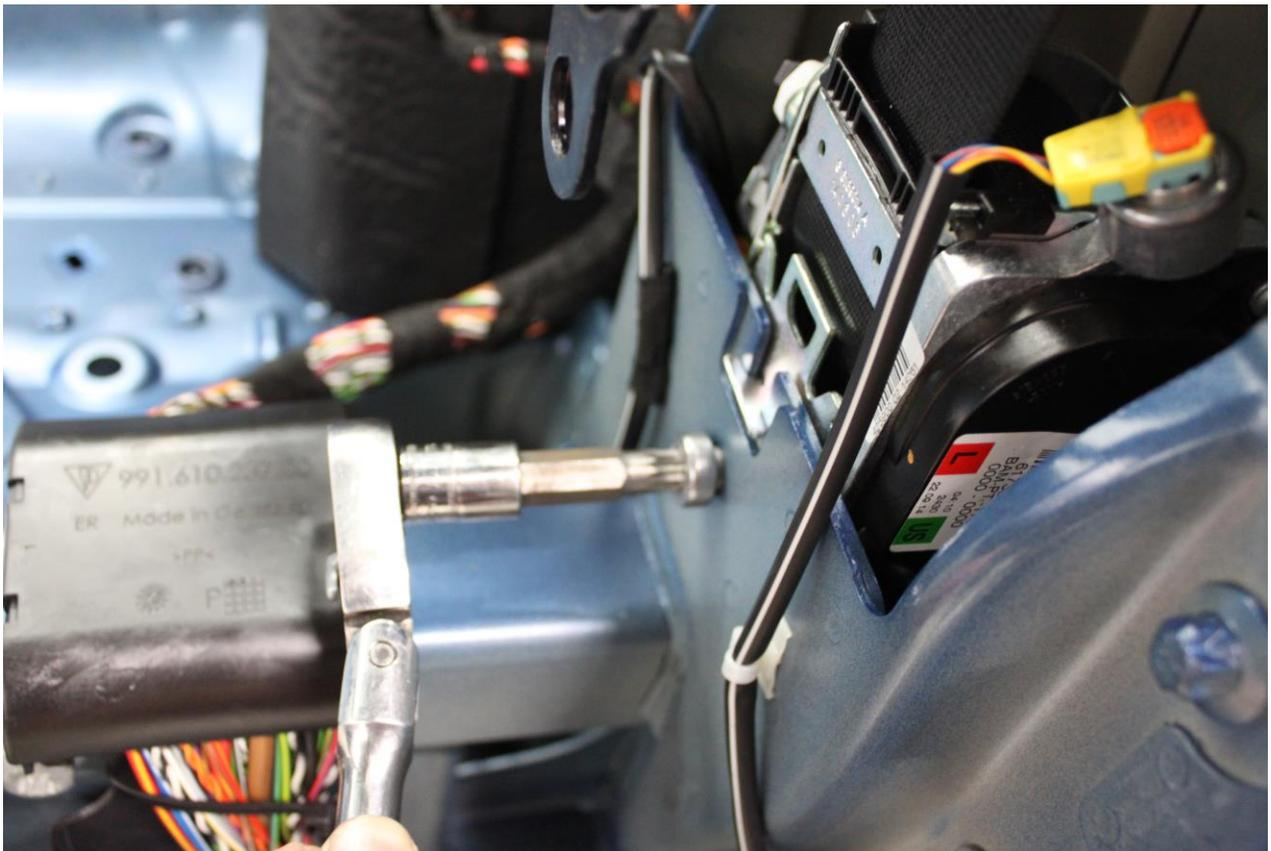
17. Remove the two through bolts to the lateral beam (16 mm bolt head)
