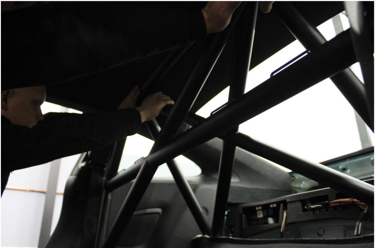
23. Align interlock connections and start all allen bolts (1/4" allen head).
