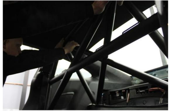
36. Starting on passenger side first, use a drift pin to help align the interlock holes. Start bolts ONLY.
