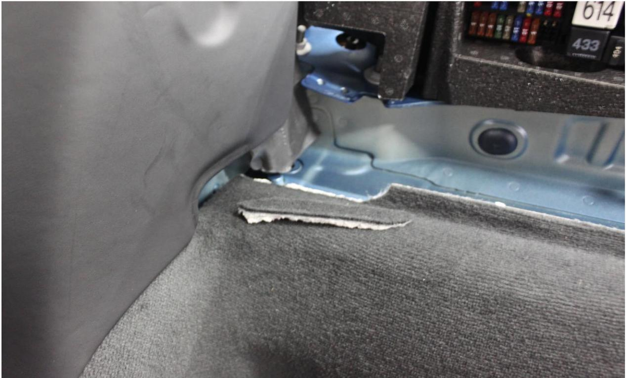
35. Using 2 people, install roll bar into car. It is a tight fit so each person should watch their side to avoid interior damage. The rear plates can be slid through the seam in the side panels where the carpet and leather sections meet to get to their mounting location. When set down close to final location the bar will need to be shoved simultaneously by both people at the top corners of the bar to get it to drop into location over the rear locating studs.
