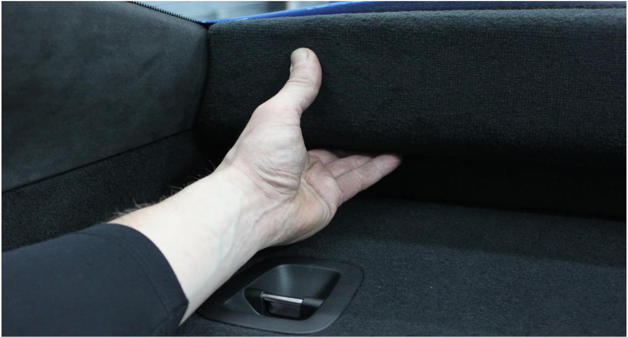
6. The upper rear carpet shelf can now be removed by first prying off the tie down point trim, then pull the piece up from the middle allowing it to fold up and out.
