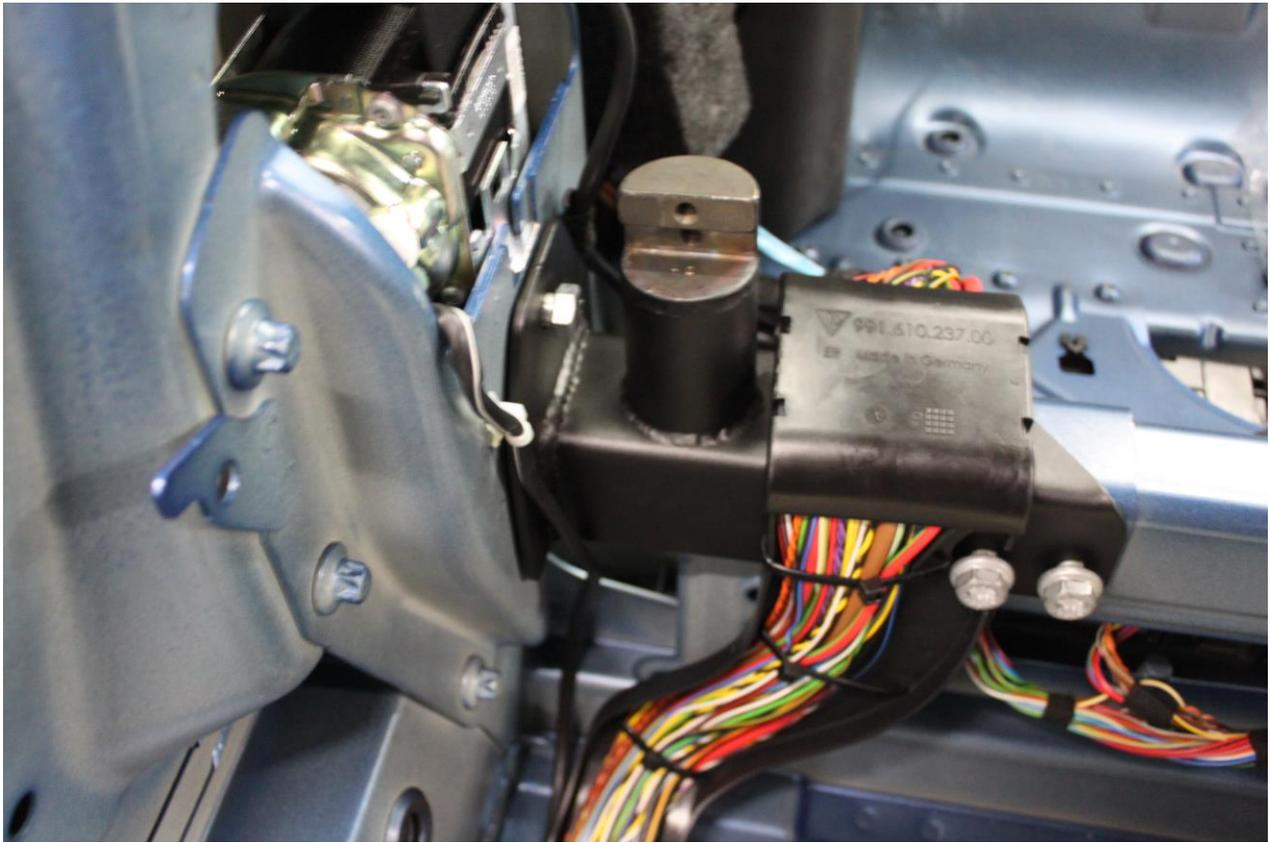
20. Be sure no wires are pinched by new base mount on sides of car. Using pliers or a knife, break off tabs on bottom of wiring harness guides to allow for a tighter fit.
