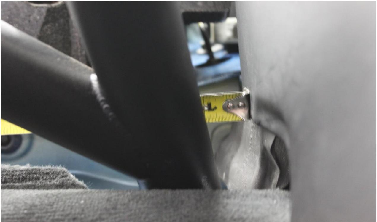
41. Draw out an oval that is approximately 1 3/4" by 3" based off of the location measurements.
