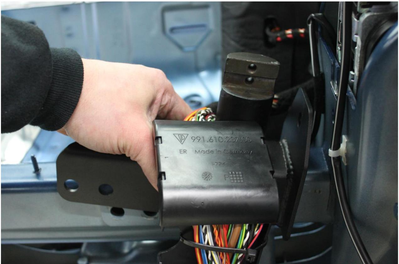
19. Use new bolts provided for the seat belt retractors at sides of new base brackets (16mm or 5/8" bolt head). (The new hex head bolts can be tightened properly since the roll bar connector blocks proper access to the factory style bolt). Start the lower through bolts. DO NOT tighten bolts yet!
