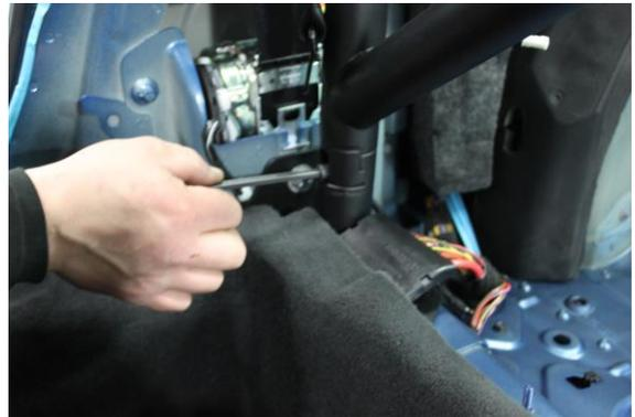
24. Make sure the rear mount bolts can be started. Tighten the allen bolts then the 3 bolts at each base mount.
