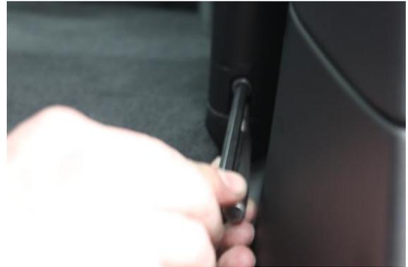
37. Next, start drivers side followed by the rear mount bolts. (Lock washer for rear bolts goes between bolt head and flat washer. Bolts are 17mm bolt head.)
