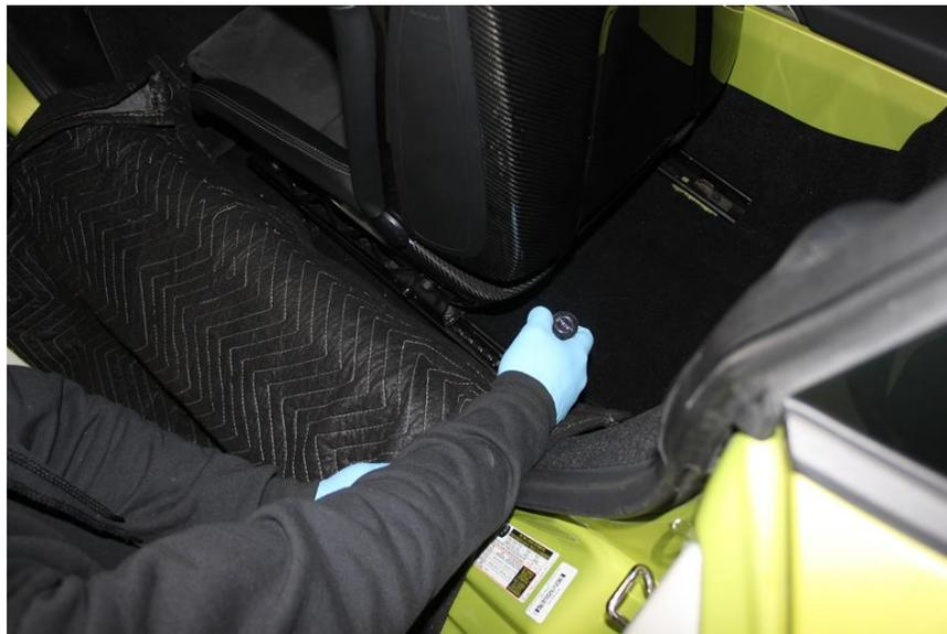
Unplug seat at large yellow connector by first releasing black lock tab, pulling it straight out.
