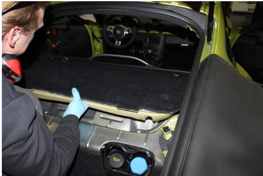
Remove silver garnish at back of engine cover by first removing two screws behind the oil and coolant fill door, then pull up firmly working from one end to the other.
