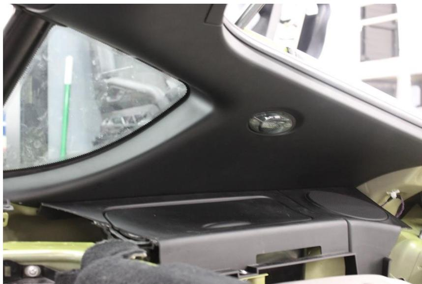
Install main hoop assembly again but do not final tighten. Be sure to put the two M8 washers between the seat belt guide pin and the body for correct
