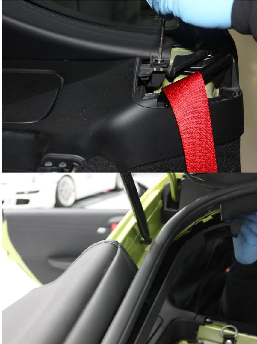
Rear speaker/strut covers can now be removed by first removing two screws at front then prying up beside the strut dome. Unplug speaker.
