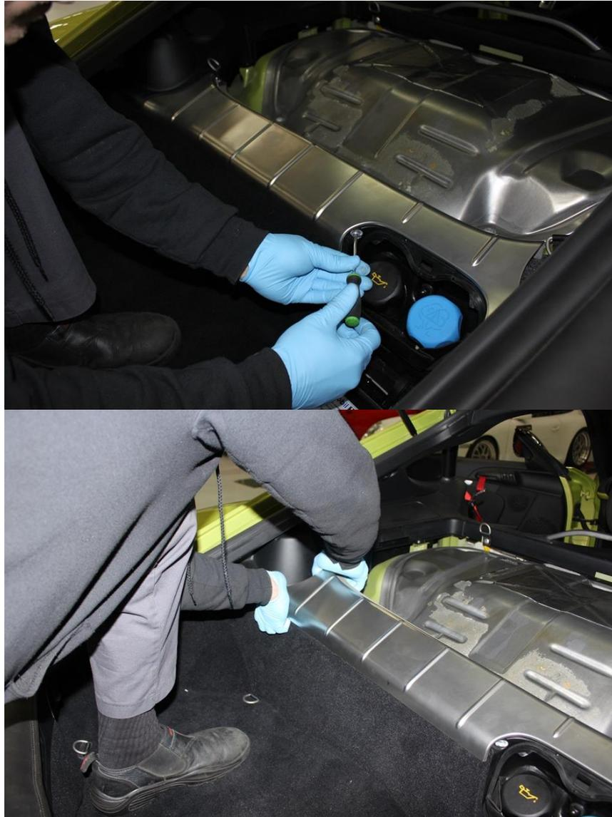
Remove upper grab bar at front of engine cover by pulling up rubber base trims to access bolts. PIC
