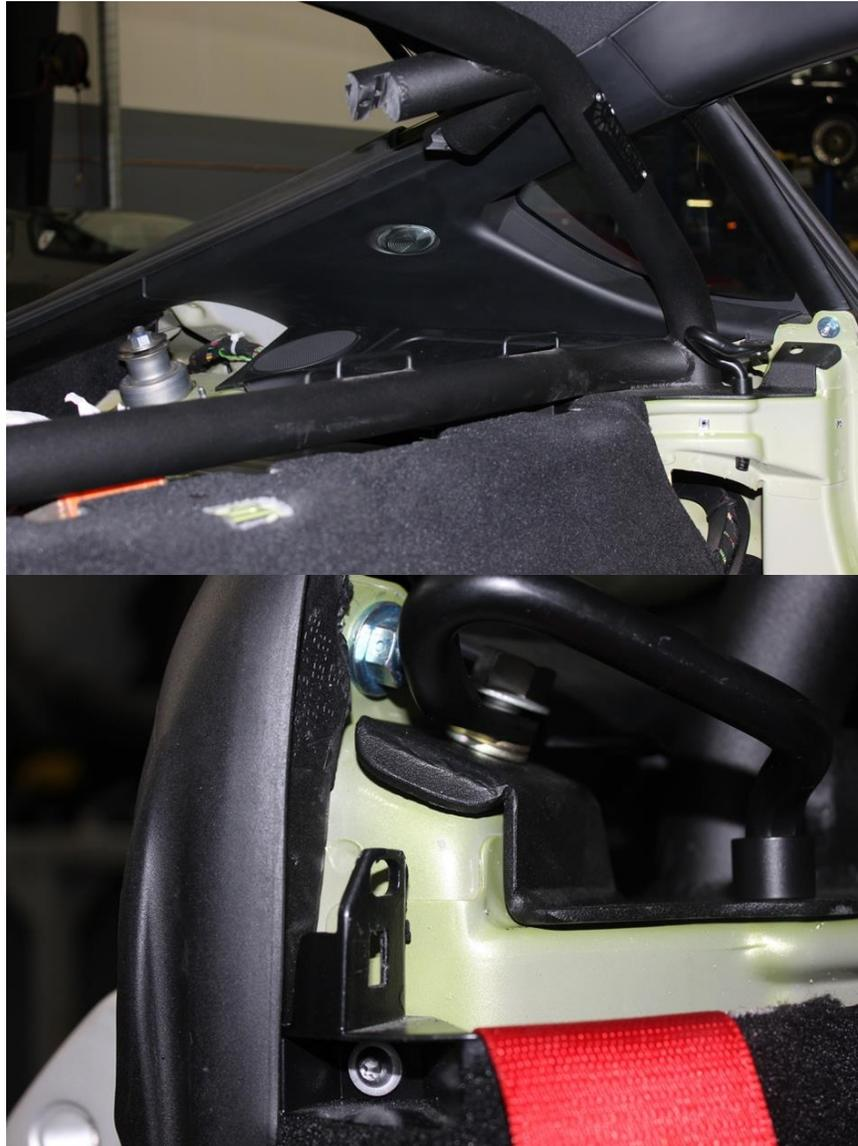
Next install rear stays and start all fasteners. Raise rear of car and set on jack stands to allow full droop of suspension. Then install new bolt for rear stays from the wheel well into the cabin and start nut. (Assistance from a second party will be helpful for this bolt.)
