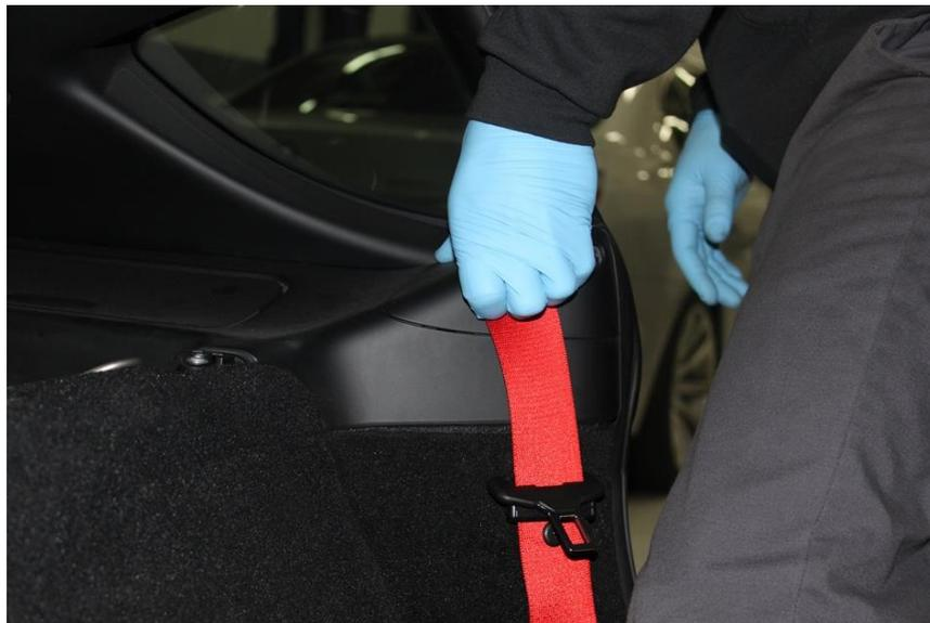
C pillar trim can now be removed by first removing screw at the lower front edge for each side. The trim piece can now be pried out by starting at the top hatch opening and pulling down. Unplug light then pull trim up and out.
